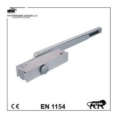
Extruded Aluminium Alloy Housing Precociously Machined & Finished Two Speed Control for Approach & Latching Jerk Free, Smooth Operation Controlled by Rack & Pinion Mechanism Universal Mounting for Left & Right Hand Doors without adjustment Suitable for Wooden & Metal Framed Doors ISI Marked as per IS 3564:1995 & CE Marked Preloading of Arm for adjusting closing force EN2-4 Inbuilt Hold Open option which helps to hold the door from 10° to 90°Tested for 5 Lakh cycles from Govt. Approved Lab
